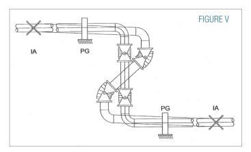
Figure V illustrates the use of a two-hinge system to absorb the major thermal expansions in a single plane "Z" bend. Since the pressure thrust is absorbed by the hinges on the expansion joint, only intermediate anchors are required at each of the piping system. The thermal expansion of the offset section containing the expansion joints must be absorbed by bending of the
